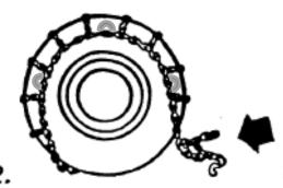
Lay chain over the tyre, cross chain hooks up and the Cam fasteners on the outside of the tyre. Tuck the spare length of chain under the tyre.
